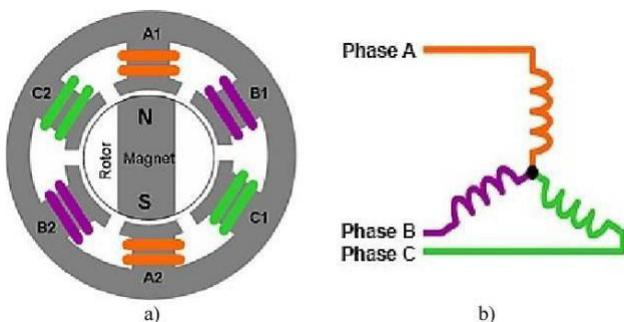
Fig. 1. BLDC motor: a) simplified internal structure; b) motor phase
